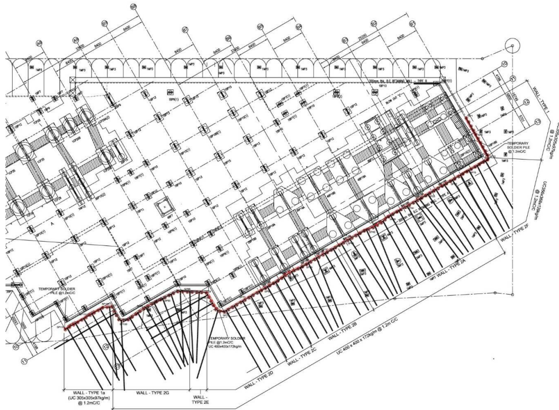
Figure 2 : Anchored Timber Lagging Soldier Pile Wall
