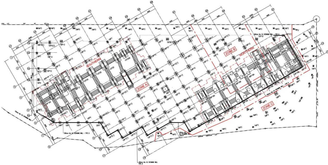
Figure 1 : Alternative Piling Layout
