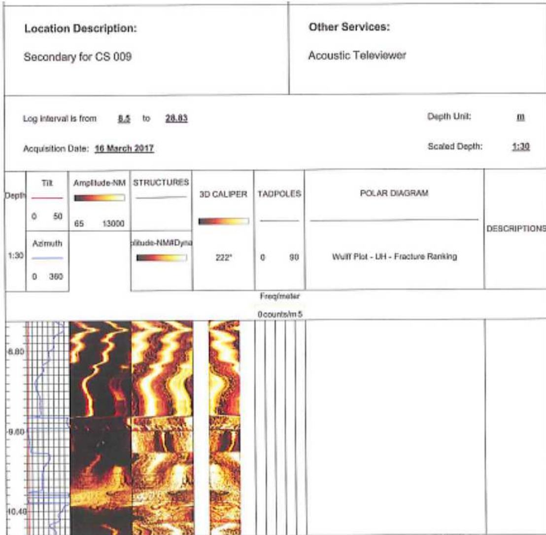
Figure 4 : Logged Cores Show Rock Mass/Joint Condition
