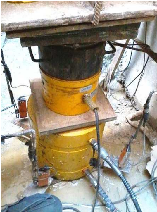
Figure 3 : Caisson Plate Bearing Load Test
