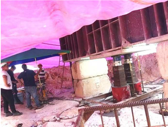
Figure 4 : Footing Plate Bearing Load Test
